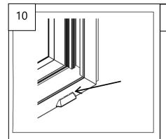
28. Run a bead of silicone around the edges of the weep flap.
